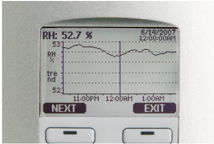
The display shows measurement trends and over four years of real-time measurement history.
