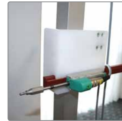
Electrical deflection sensor provides accurate results about the deformation of the test block.
