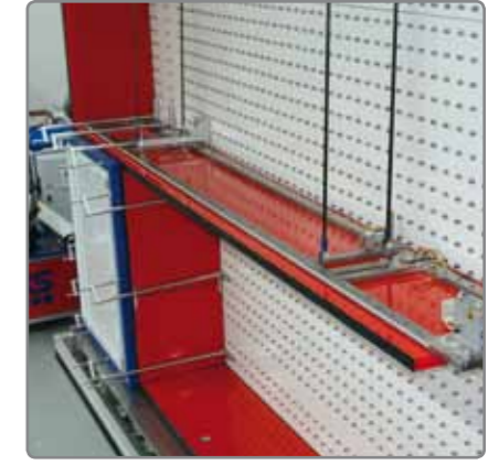
The upper test chamber cover can be positioned easily and is also available with motor drive*.
