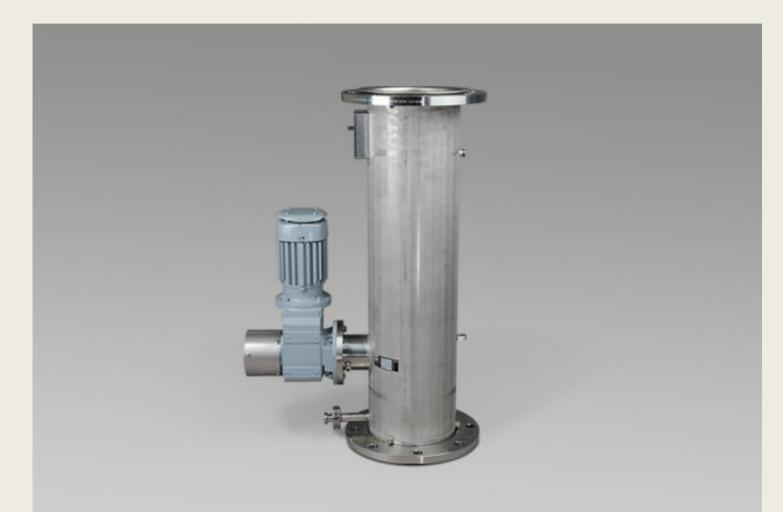
TWISTER 200 with sample outlet for on-line measurement | Suitable for process lines with a diameter of 200 mm (DN200) and for combination with in-line MYTOS | ATEX and GMP versions optionally available
