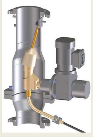
The principle of dynamic sampling is the same for all TWISTER models. When a signal is received from the analysis system, the probe tip traverses the entire pipe cross-section on a spiral path with a constant speed in order to achieve equally weighted sampling. The TWISTER scan starts from a protected parking position and moves across the cross-section in the spiral pattern around the center of the pipe, passes through the center axis and runs back to the parking position.
