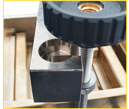
Quick release of the crossbeam to remove the shear box, optimizing assembly time.
