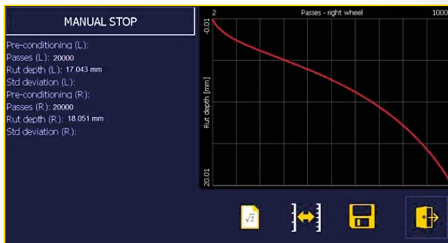
Test execution and all parameters, such as water/air temperature, specimen temperature, rut depth can be monitored in realtime. The software also allows exporting test data to an Excel compatible format
