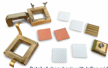
Detail of shear box's with teflon grids
