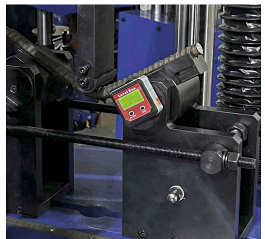
H001B-41 this jig is equipped with inclinometer
