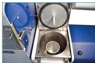
Cup into the centrifuge, up to 8000 revolutions per minute
