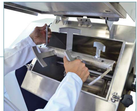
Detail of the detachable mixing shaft with helical blades
