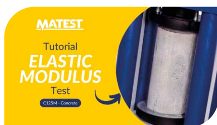
How to Perform an Elastic Modulus Test on Concrete EN 12390-13 | ASTM C469
